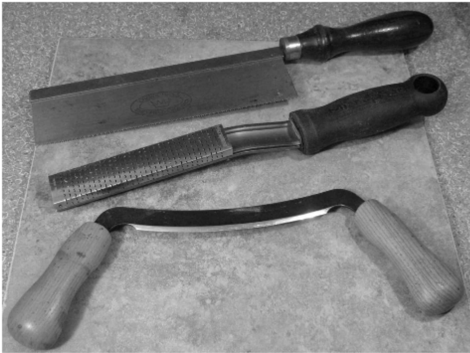
Pictured here from top to bottom are a fine-toothed handsaw, a microplane, and a curved drawknife.
