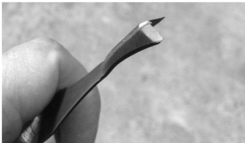
Here's what a V-tool looks like close up. There are two razor-sharp cutting edges that meet in a point.
