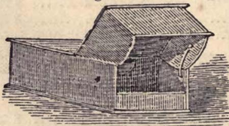
ballots. The front of the box in which the ballots are placed is opened, as shown in the engraving; the ballots are then deposited in the rear through a convenient opening in the partition. During the process of voting the hand of the voter is completely screened from observation, thus rendering the balloting entirely secret. After
