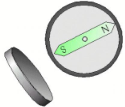
Using a compass to identify the pole of a magnet.
