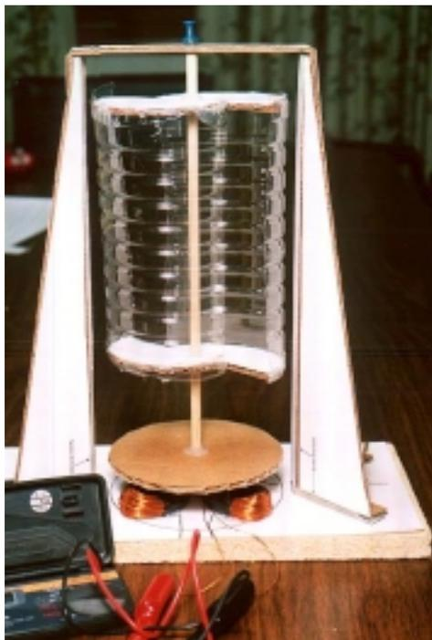
The completed vertical axis turbine.
