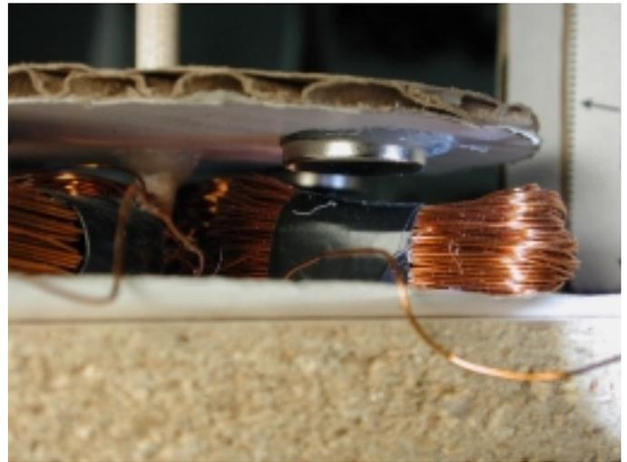
The magnets should pass as close to the coils as possible.
