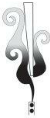
Fig. 45 – Effect of flute on the surrounding air
