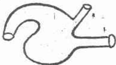
I had a retort made with two tubes, one in the center and one below at the bottom, as the figure shows. Through tube (a) I let the water drop in as indicated in the previous process, and quickly closed the hole up. After that, I directed the bellows into tube (b), and as soon as the cold water had dripped inside, I worked the bellows. An observer would have had great fun seeing how frequently
