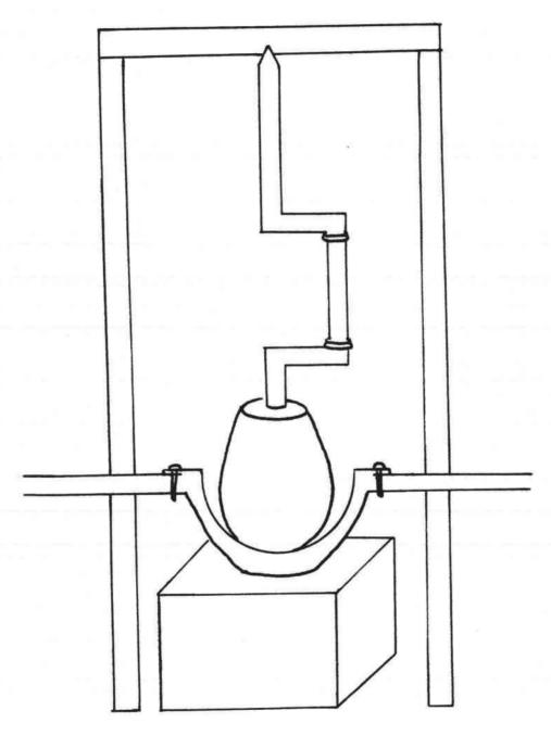
The mortar must be made of Cast iron and must be turned in the Inside and polished. The pestle the Same must be turned off on the outside. This Labour of amalgamation, whether it is done with the Engine or with the hand only in a mortar, must be continued a good while, and the aaa must after that, be washed So long, until it yields no more blackness, but appears as bright as a Looking glass.
