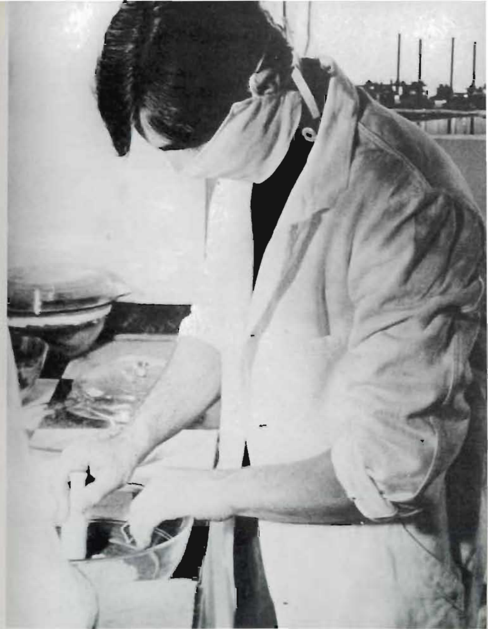
Sifting. To eliminate the impurities which have found their way into the plants and have not been reduced in incineration, the ashes are sifted. A mask is worn, because the salts they contain are very volatile and can be harmful.
